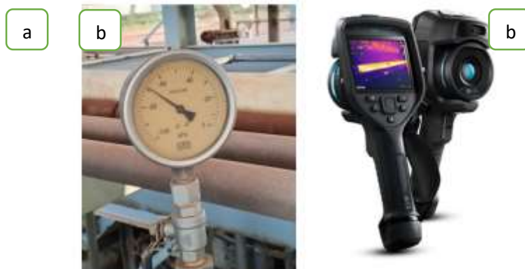
Figure 1 : Instruments used for data acquisition: (a) SA GAUGE vacuum gauge; (b) FLIR E96 infrared camera.
