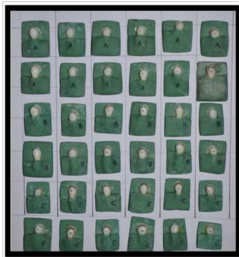
Figure 2: Tooth mounted vertically in chemically cured resin with the buccal cusp stabilized for measurement.
