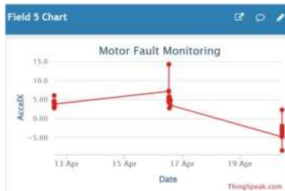
Fig.6. shows the Motor fault monitoring showing vibration variations in ThingSpeak.
