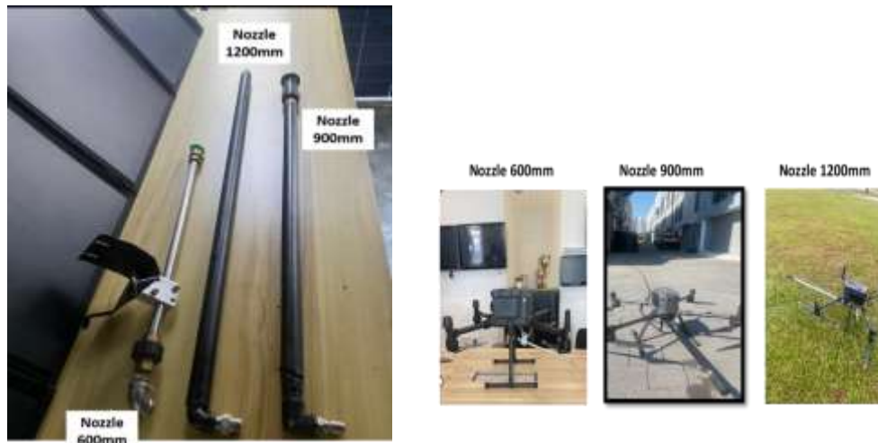
Figure 3: Comparison of the customised spray nozzle configurations evaluated during the experimental programme.
