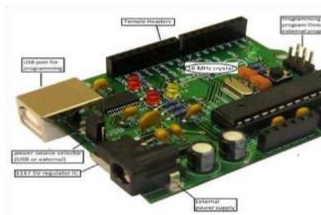
Fig4.2 ArduinoBoard Starting clockwise from the top centre:
