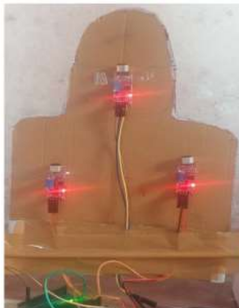
Figure 10 shows how the sound sensor is positioned behind the target.
