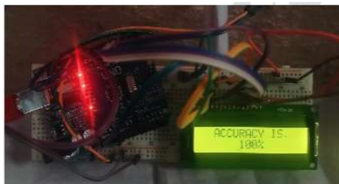
Figure 4: When the bullet is within 100% of the range, a message is displayed.
