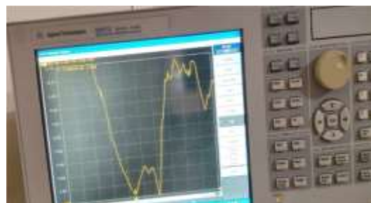
Fig4.19 Measured VSWR on Vector Network Analyzer
